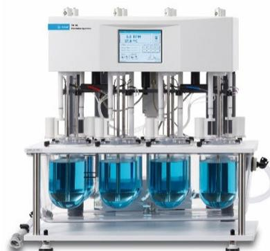
**Note:** It is important that the heater/circulator is full of water prior to applying power or it may damage the heating elements in the circulator.
