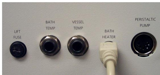
Ensure that communication cables to the apparatus are restored to their proper locations as indicated on the rear of the drive unit of the apparatus. Similarly connect any other equipment, such as an autosampler, to restore the desired configuration. Lastly, connect the power cable to the jack in the rear of the apparatus drive unit and plug into the power source.
