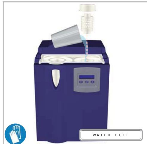
Fill the water bottle using fresh deionised water to a level approximately 15mm below the upper lip of the neck of the bottle. If the generator is powered up an audible and visual indication will be given when the correct level is reached.
